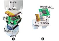
Figure 3: InSight Hardware: a) the G-Sens IR receiver; b) the G-Ripple IR laser.
