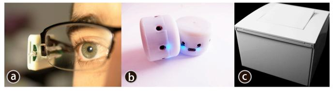
Figure 1: The InSight hardware components: a) the G-Ripple clip-on IR laser source; b) the G-Sens sensor to augment existing objects; c) example controller augmented with the hidden G-Sens sensor.
