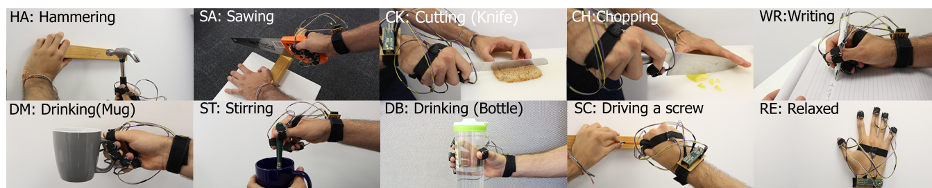
Figure 1: OSense propose a new technique to identify object-activities by using motion data and posture data. This figure shows the object-activities used to evaluate OSense.
