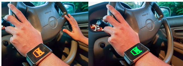
Figure 4: Self-awareness app for drivers: Samsung Gear Live smartwatch with CompRate model provides feedback when the driver needs to rest. To get initial feedback, we developed an app which provided HRV feedback every 5 minutes.
