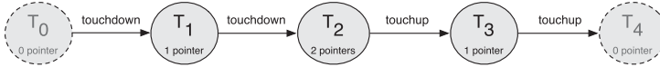
Fig. 8. The state transition diagram for the two-finger Tap gesture in Figure 7. T_1 , T_2 , and T_3 are specific to the gesture, whereas T_0 and T_4 can be shared by other gestures.
