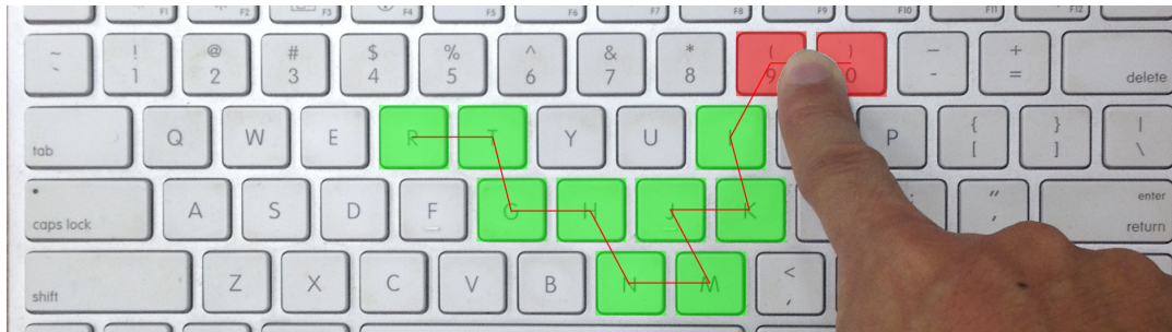
Figure 1: Gesturing on a physical keyboard. The green overlays show the keys that have been pressed and the red ones show the currently pressed keys. The red line running across keys illustrates the captured gesture stroke.
