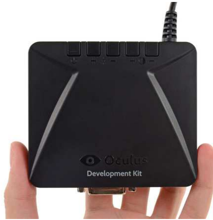
Figure 2.15: Oculus Rift control box showing brightness and contrast adjustment buttons.
