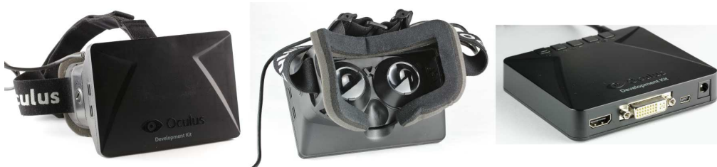
Figure 1.10: Oculus Rift head mounted display. Left: front view. Center: back view. Right: control box.
