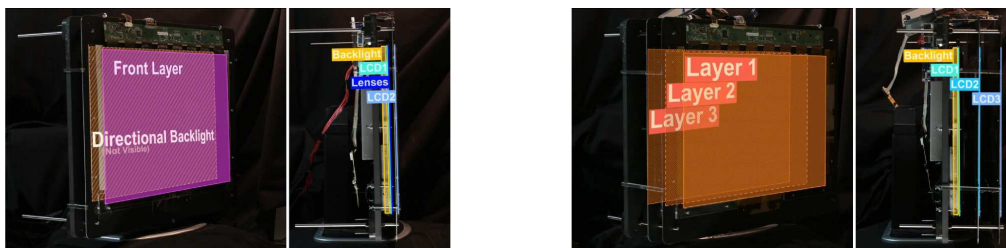
Figure 1.8: Two prototypes of light-field display built in MIT [115]. Left: a directional backlighting setting. Right: a multi-layer setting.
