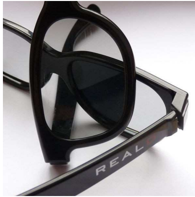
Figure 1.3: RealD polarization glasses, demonstrating the opposite polarization between the two eyes' filters.
